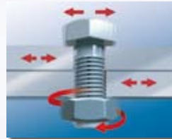
Vibration and loosening
